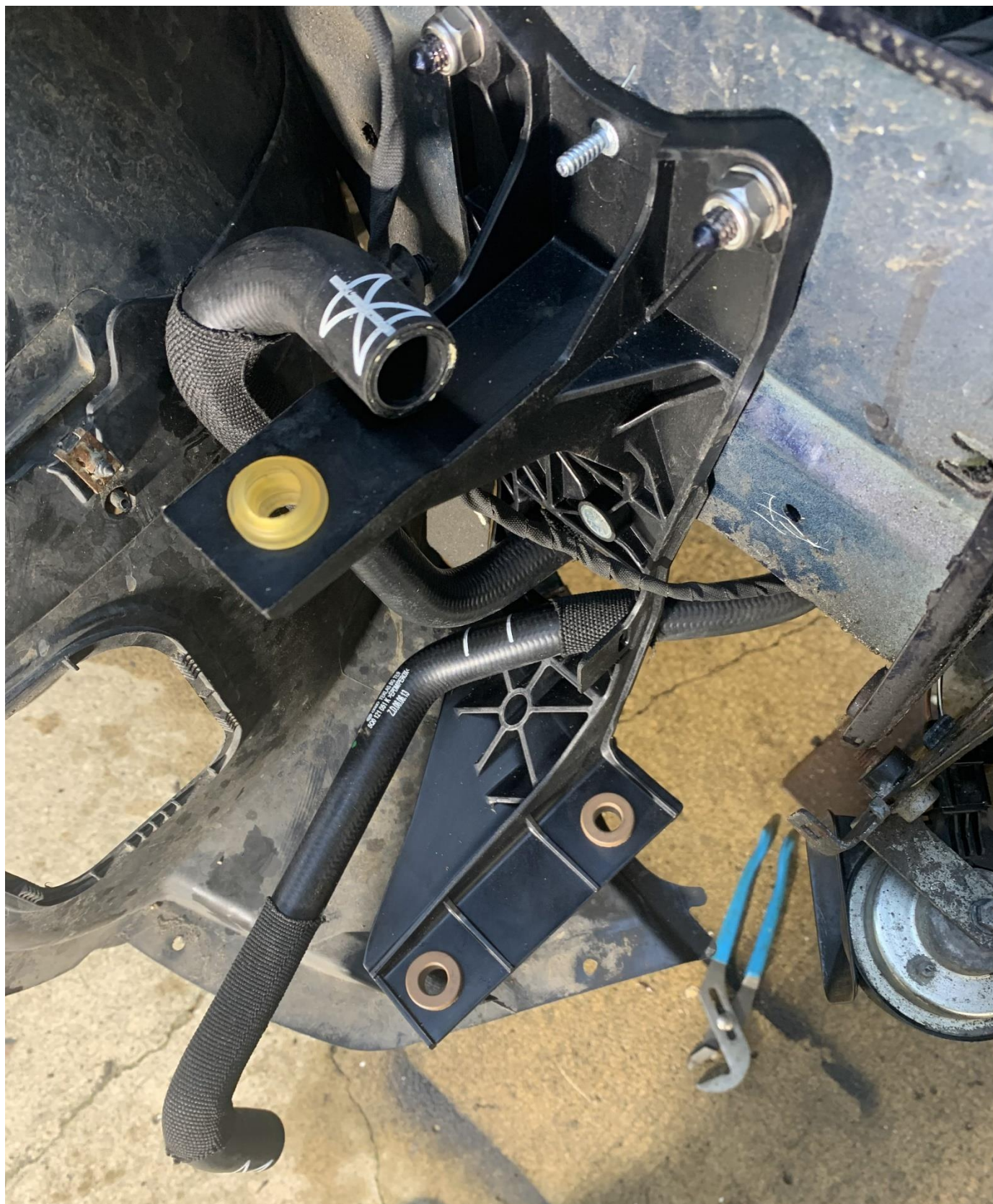
RHS Aux Cooler Mounting Bracket: 5Q0121093FD (#24) Installed
