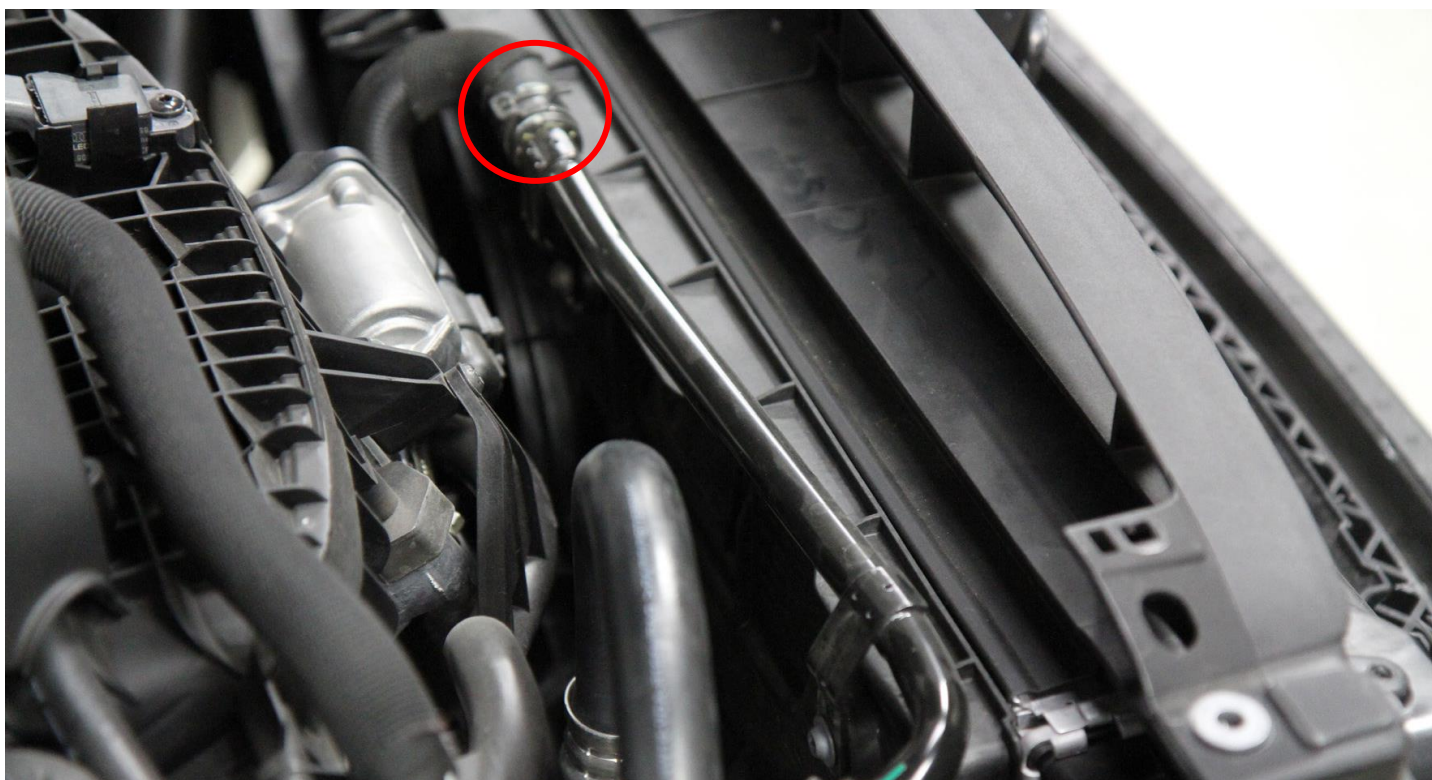
Coolant Pipe: 5Q0121070AP (#26) & clamp N90686902 (#61)
