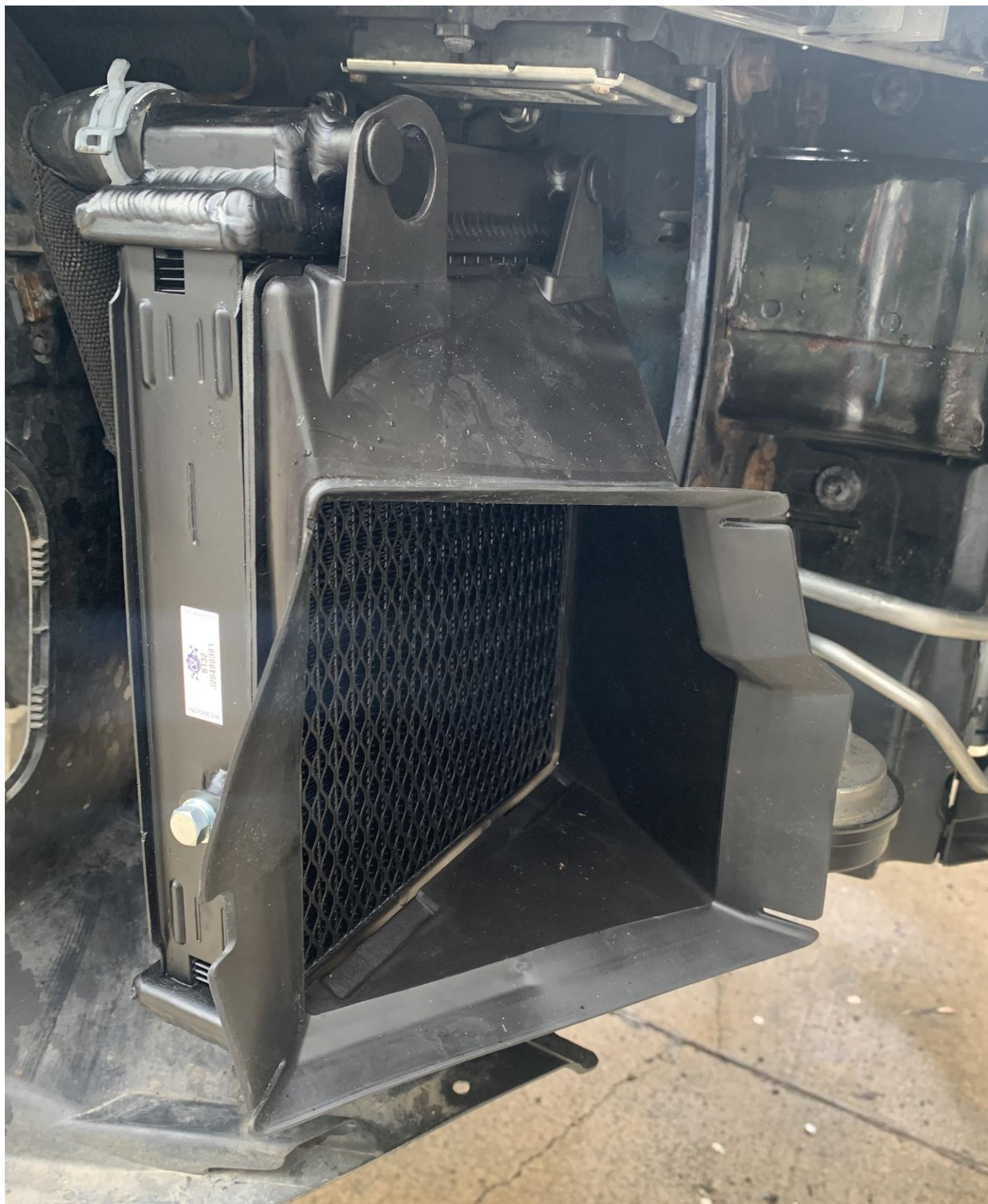
CSF #8132 Aux Cooler Installed with Air Duct 5G0-117-334 (#31)
