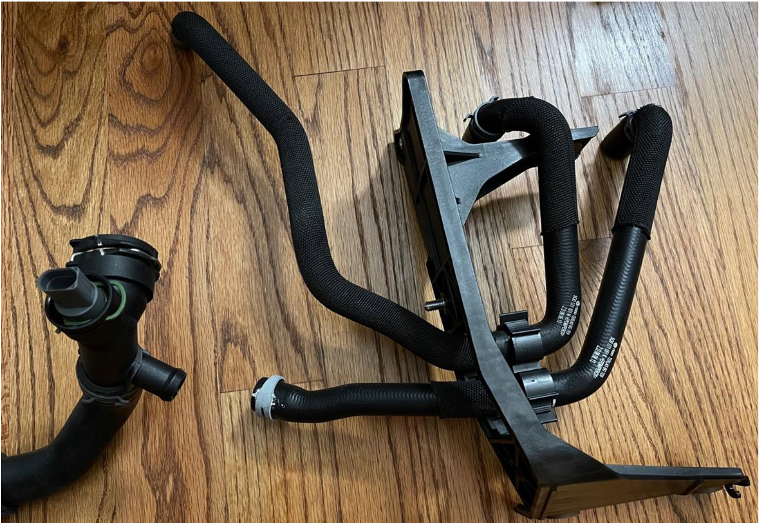
Lower Coolant Hose: 5Q0122051EG (#1) & connection to Hose 5Q0121051K (#21)
