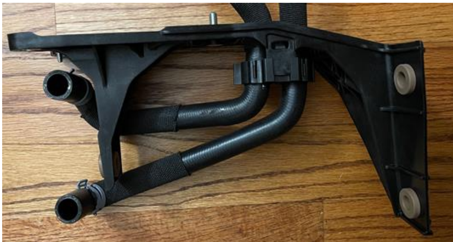
Hose Separater Bracket: 5Q0121093BD (#27) & Rubber Grommets: 4D0317867A (#25)
